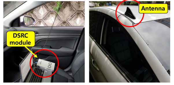
Fig. 9. DSRC module and antenna setting for the real-world experiment.
