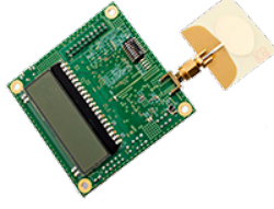
Fig. 7: UWB Transceiver based on Qorvo DW1000 radio.
