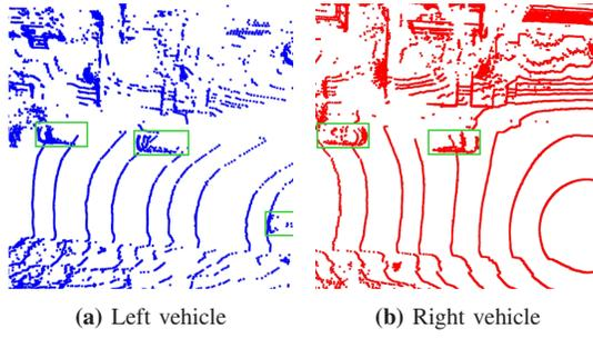
**Fig. 2:** Point cloud with the optimal selection distance for each vehicle
