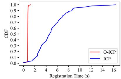
**Fig. 5:** Comparison of registration time between O-ICP and ICP
