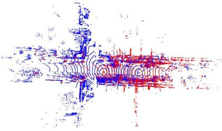
**Fig. 4:** Registration result of the point clouds from two vehicles.
