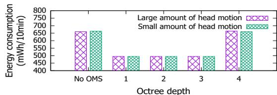
Figure 1: Impact of octree depth  $d_O$  on the Hololens energy
